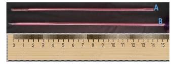
Fig.1: The conventional intramedullary pin Kirshner pin (A) and the improvised long screwdriver pin coated with chrome vanadium (B).
