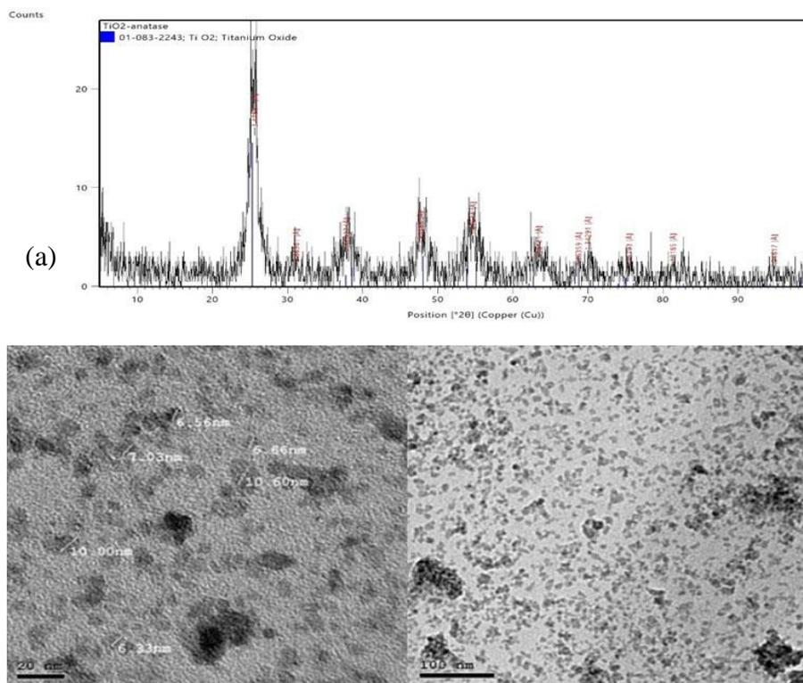
Fig. 1: XRD pattern of the prepared TiO<sub>2</sub>-NP (a) and TEM images of the prepared TiO<sub>2</sub>-NPs (b).
